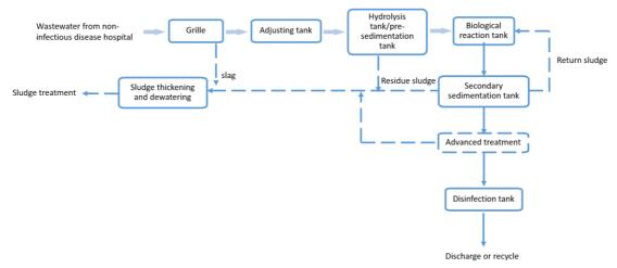
**Figure 2.** Secondary treatment for non-infectious disease hospitals (wastewater can be discharged into surface water, sea, or recycling).
