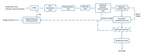
**Figure 3.** Wastewater from infectious disease hospitals require pre-disinfection, secondary treatment, and disinfection treatment.
