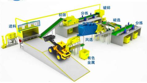
Picture: Illustration of the CDW treatment system
